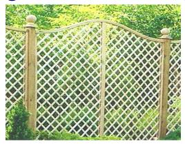
30x35mm Frame, T&G joints, 6x20mm laths, rounded edges.
